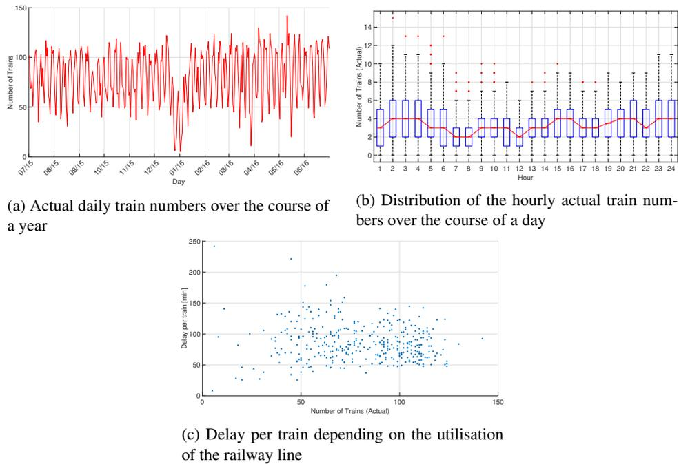
Figure 10: Traffic and delay pattern for a freight train line
