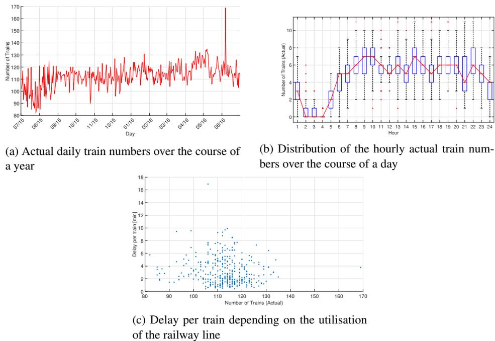
Figure 11: Traffic and delay pattern for a mixed traffic line
